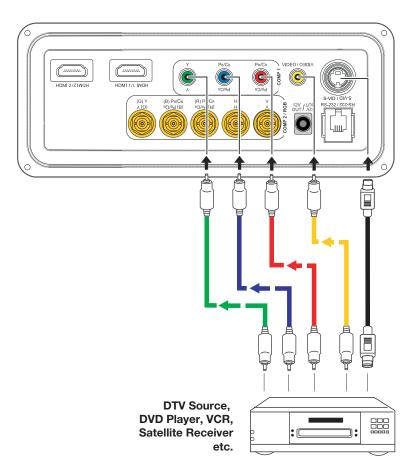
Figure 3-13. Composite, S-Video and Component Video Connections
